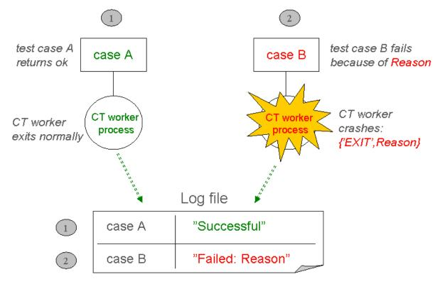
Figure 3.1: Successful and Unsuccessful Test Case Execution
